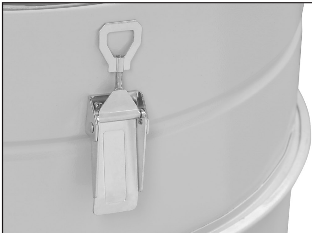
Figure 35. Collection drum lid latch installed.
